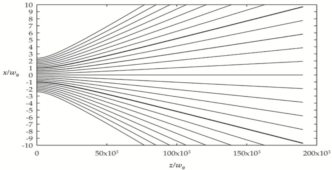
De Broglie's wave trajectories and waist lines on the symmetry  $(x, z)$ -plane for a *Gaussian* beam with waist  $w_0$  and  $\lambda_0 / w_0 = 2 \times 10^{-4}$ .
